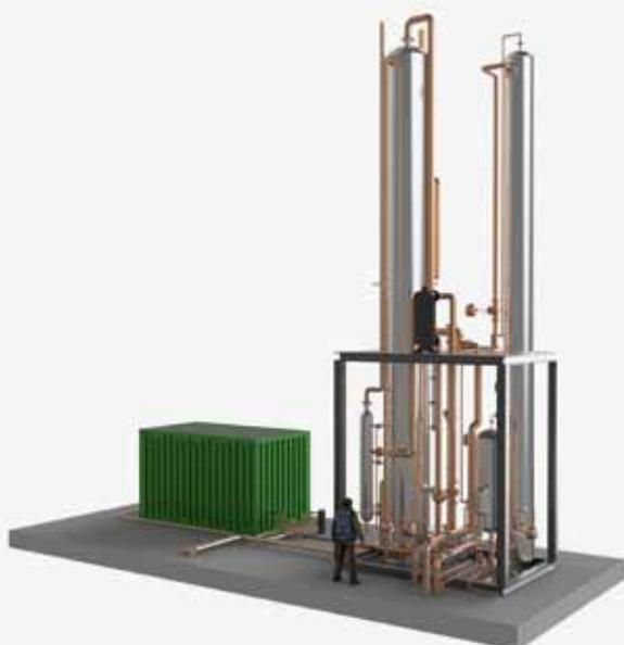
*GM has built an upgrading plant for the treatment of 200 Nm<sup>3</sup>/h OFMSW. The unit will produce high-purity biomethane, in accordance with the limits laid down by the SNAM network code and with the UNI TR 11537 regulation. The pre-treatment section, operating at atmospheric pressure, allows to remove the undesired elements from the biogas, guaranteeing the requested technical standards for the biomethane and the values provided by the Legislative Decree 152/2006 about tail gas.*
