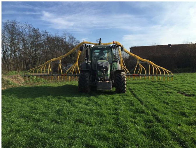
Figure 10 - Digestate is injected into the soil using an 'umbilical cord' to avoid soil compaction
