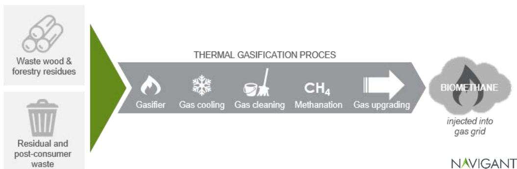
Figure 8 Schematic overview of the thermal gasification process
