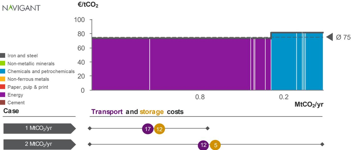
**Figure 60** Marginal carbon capture costs for Porto Marghera, totalling 1.8 MtCO<sub>2</sub>/year at a weighted average capture cost of €75/tCO<sub>2</sub>. Transport and storage costs differentiated based on CO<sub>2</sub> flow rate.
