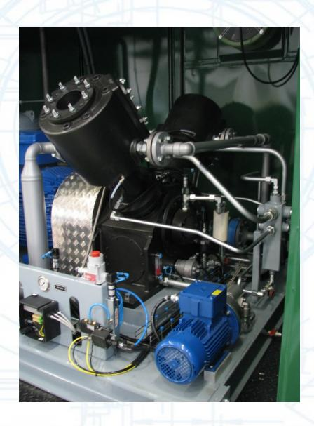
Application: gas injection Inlet pressure: 4,5 - 6 bar Outlet pressure: 21 bar
