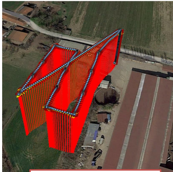
Drone path 40 m height flight test
