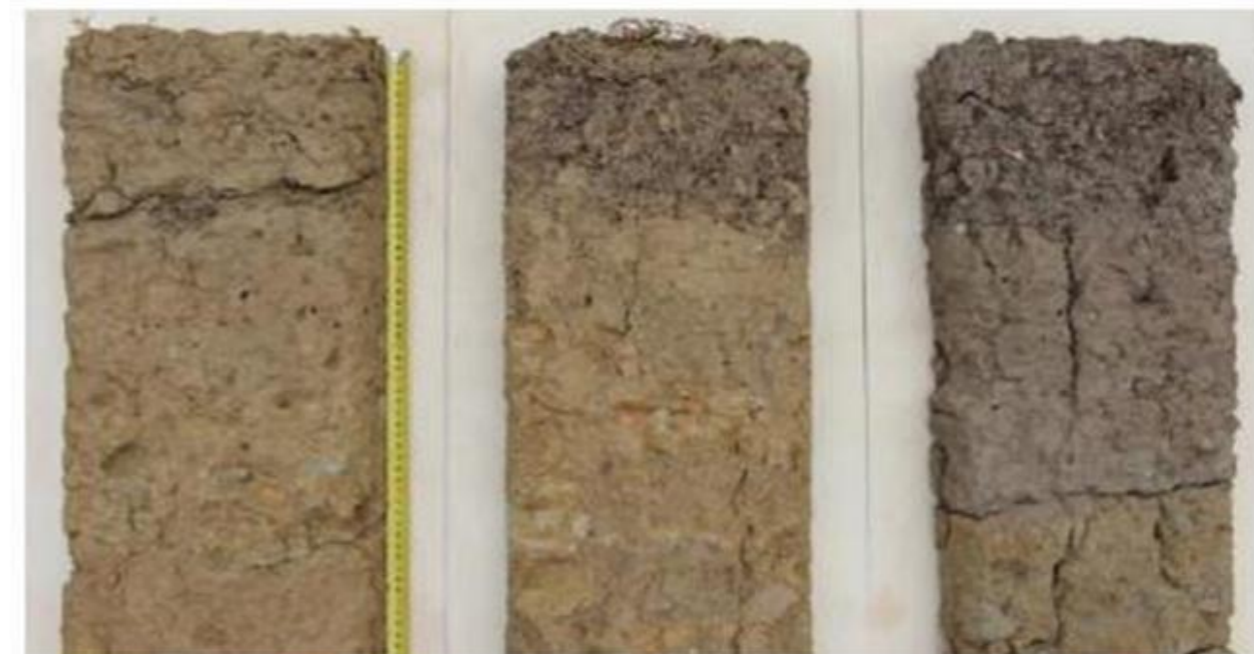
Carbon increasing in soils: left: start, middle: after two years, right: after 5 years
