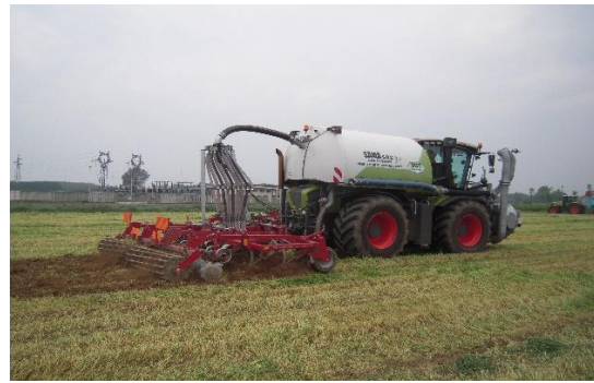
FIGURE 8 A) DIGESTATE INJECTION SYSTEMS: OPEN SLOT SHALLOW INJECTION ON THE LEFT; B) CLOSED SLOT SHALLOW INJECTION ON THE RIGHT (SOURCE: CIB – CONSORZIO ITALIANO BIOGAS)
